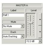
**Level:** allows lowering a corresponding channel's level by a value of up to 90 dB. Setting is possible via soft fader or using the UP/DOWN buttons.
